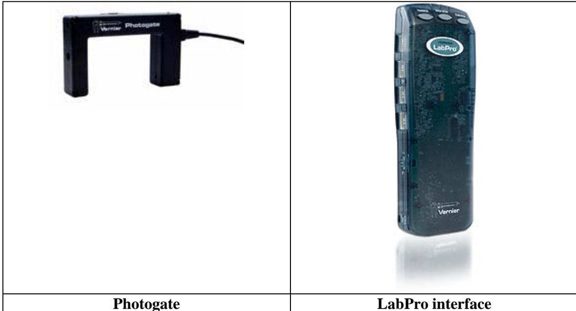
Make sure that the lab Pro interface is plugged into an AC outlet and is also connected to the USB port of the computer. Connect the photogate to the DIG/Sonic 1 port of the lab Pro interface.
